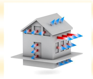
In the same way that we can add layers to keep us warm, most homes can be insulated to slow down the loss of heat and thus keep you and your home warmer for longer on cold days. Insulation can be added to walls, under floors and in roof spaces.
